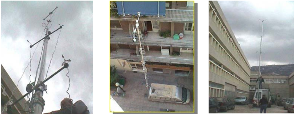
Fig. 1: Measurements with the mobile meteorological station and the telescopic mast.
